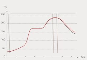
Multi Vacuum Technology enables up to three vacuum steps per soldering cycle.
