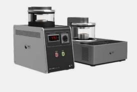
The Ion Sputter Coater allows for imaging of nonconductive samples in high vacuum mode for the highest resolution imaging. Sputter coaters increase conductivity by coating the test specimen with a few nanometer thick metal film of Au or Pt. The higher conductivity increases the amount of secondary electron generation and creates higher resolution images.
