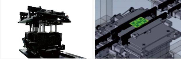
4 ball screws with high precision & stiffness and additional 3 shafts.
