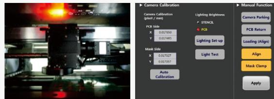
Camera X and Y axis driven & controlled by ball screw and Servo
