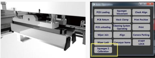
Cylinder and Motor driven printing head makes an uniform printing result.
