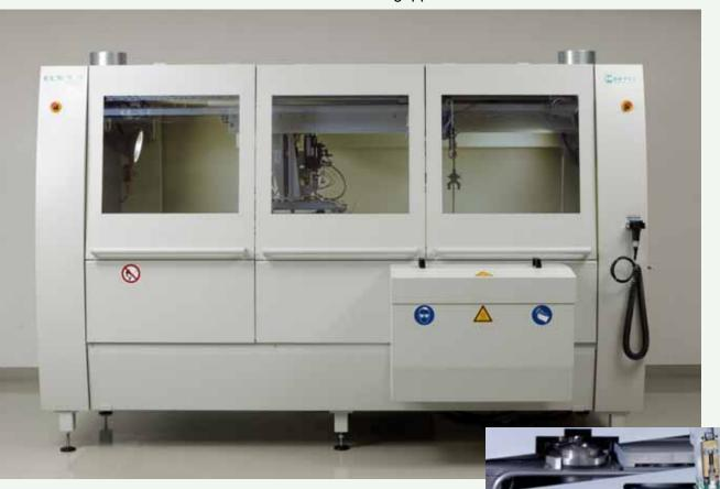
the inline design of the indivdiual components, fluxing, pre-heating and soldering, 3 pallets can be processed in the system and the processes managed separately from each other in a cycle-neutral manner. A pin chain transport is installed above the fluxer and the pre-heating system for this purpose. A 40-mm soldering wave can be used for soldering work on small subassemblies.
