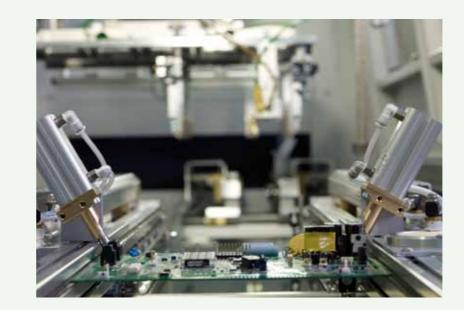
The ELS 3.3 soldering system has been designed for the production mix of small and medium series. The easy-to-program miniwaves with wettable and contraflow nozzles enable any subassembly to be processed using optimized parameters.
